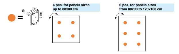
Description of the structure and ceiling fixing kit:
