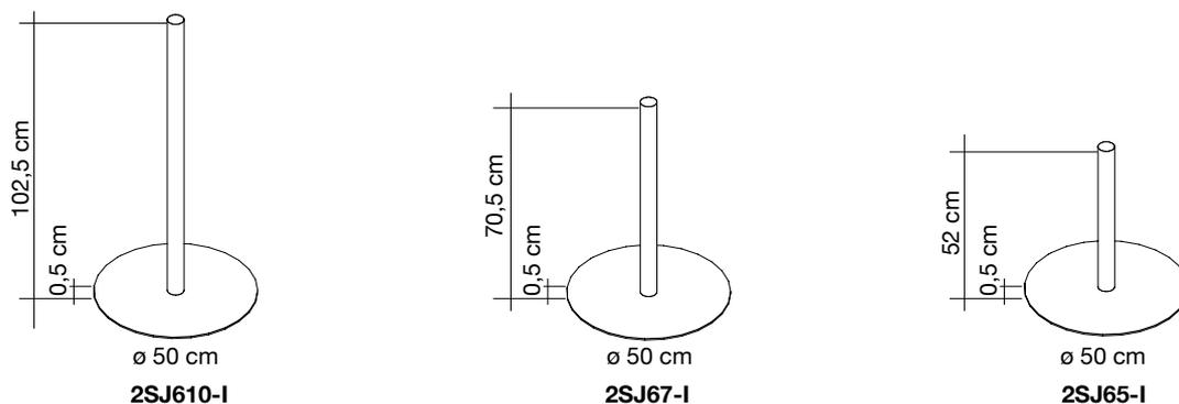
Strutture per tavoli cod. **2JV610-TI, 2JV610-SI, 2JV67-TI, 2JV67-SI, 2JV65-TI, 2JV65-SI**
