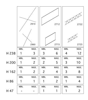
Minimum and maximum number of load bearing elements for a complete module.
