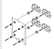
Wall-mounting with screws and spacers for codes: 5130, 5131, 5134, 5135, 5138, 5139, 5185, 5186, 5143, 5153
