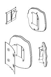
Wall-mounting with a steel plate with a double-sided adhesive for
