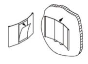
Wall-mounting with double-sided adhesive for codes: 5129-BA
